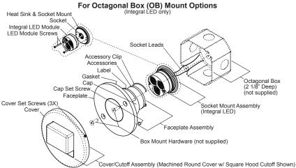
connectors (not included) per applicable codes. Note: Be sure that the power being supplied matches the rating on the fixture Label.
